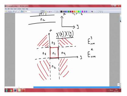
So, I can take a waveguide like this as a certain refractive index and now if I want to dissociate into different components so let me say this is y axis and this is x axis. So, if I look at this then what I see here is I can have region n1, I could have multiple possibilities here, and I could have n2 here and that could be n3, it could be n4 and n5. So, these are all the different regions or different boundaries that we should consider when solving for a waveguide here.
