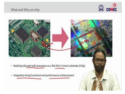
So, integrated circuits or integration on-chip has been a philosophy for microelectronics over the past couple of decades. So, the whole idea of integration coming from realizing bulk functionalities. So, you have various components that you see on the left side, there is an oscillator you have passive elements resistors and capacitors all in a circuit board. This is a printed circuit board.
