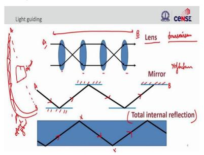
So, in order to understand how to convert this lenses and mirrors into circuit let us look at how do we guide light so we have to make sure you take a photon or light from point A to point Be, so we want to understand how we can do that. So, we can easily do it by using lenses series of lenses and that is the example that you have here. The cartoon there shows you how one can take a lens and then arrange it in series so that you can you know take light from point A to point B.
