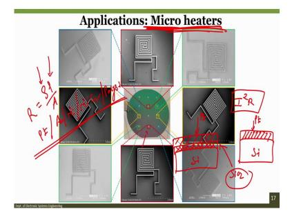
Now let us see another application of the micro-fabrication technique. Another application is in heaters. And when we say heater, we are talking about microheater. Now, what is heater? If you have a resistor and if you heat the resistor by applying a power, then your heat will I square R, which is your joules heating.
