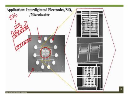
Now, let me take another example. So now if you want to have two layers on the same wafer, that means you want to have microheater on the silicon substrate, on the oxidized silicon substrate, like I said, we cannot have a microheater directly on silicon, it will short. And then over that what we want? We want insulating layer like this and on the insulating layer, we want to have interdigitated electrodes.
