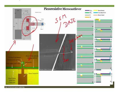
What is a thickness of this piezo resistor? So the thickness of this cantilever, thickness of the cantilever is 2 micrometer. What is the thickness of SU8, this is a tip, SU8 is about 10 micrometers. Now SU8 is very light compared to silicon, that is why it is not bending. And, of course, we have taken care of the stress effects by using silicon nitride. We will discuss it separately. And this is created using a technique called DRIE.
