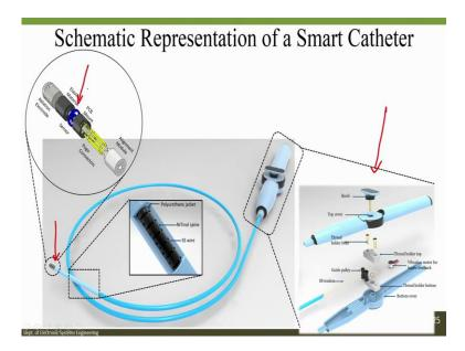
You see this is the maneuvering mechanism. You can maneuver the catheter; you can move the catheter with the help of the maneuvering mechanism. Now when you maneuver the catheter, this tube will go all the way inside the heart, and this is the tip where you apply the RF frequency to ablate. Within this tip, there is a sensor which will measure the force from the heart tissue.
