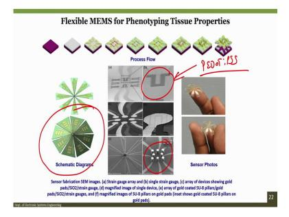
We can also create a flexible sensor, flexible microsensor. And flexible microsensor has a strain gauge, we can see here, a strain gauge. This strain gauge is fabricated using PEDOT: PSS. PEDOT: PSS is a polymer which is piezoresistive in nature.
