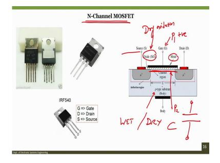
I will not go into detail about this device and how to fabricate it. The fabrication will be a separate module. So if you see this particular device, what we see here? We have a N-channel MOSFET. What is MOSFET? Metal oxide semiconductor field-effect transistor.
