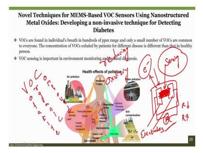
Now let us understand another area of fabrication and that is on the gas sensor side. So gas sensor is a sensor. Let us say you have electrode, and you have a sensing material over these electrodes. So here you can measure resistance.
