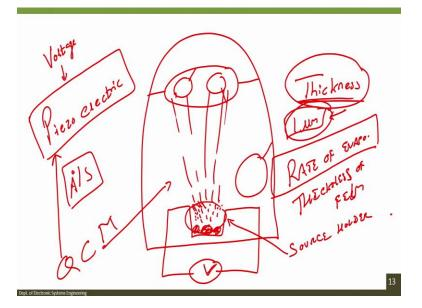
Now, if you know the rate of evaporation that means that when you open the shield when you open the shield, then this will start depositing, when we start depositing what will happen? When we start depositing what will happen? That the substrate, that will be deposit on the substrate. Again we want to stop after we reach 1 micron.
