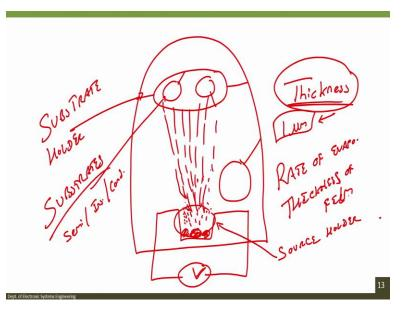
So, now you have a chamber and here you have your substrate holder and on this substrate holder you have loaded let us say two silicon wafers. And then this is your metal, let us say it is aluminum and you are going to heat this source holder by applying a voltage V. Now, when you start heat, when this source holder starts heating this will start melting and it will start evaporating.
