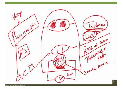
So, to show stop it as soon as it reaches 1 micron we will again put the silt back so that even this because you see when it is at high melting point it will not suddenly cool down, it will take some time to cool down if we make the voltage we bring the voltage back to 0, from let us say 100
