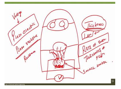
So, there are, before we open the shield, before we open the shield, there is a quartz crystal on which this deposition will occur along with the shield and this quartz crystal will tell you what is the rate of evaporation. How it will tell you what is the rate of evaporation? Because if you know quartz is a piezoelectric material. Now, see sometimes I ask very simple questions even in the interviews and people are confused between piezoelectric and piezoresistive. What is the difference?
