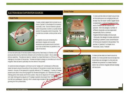
So, let me go to the next one. Now, when you talk about electron beam evaporation you should also know the electron beam sources. So, you see the first source which is shown here it is called single pocket source and a water cooled copper block is bored out to have a pocket in the shape of invented, inverted truncated cone and you can see here that it goes like this and further it goes like this that is why it looks like a cone.
