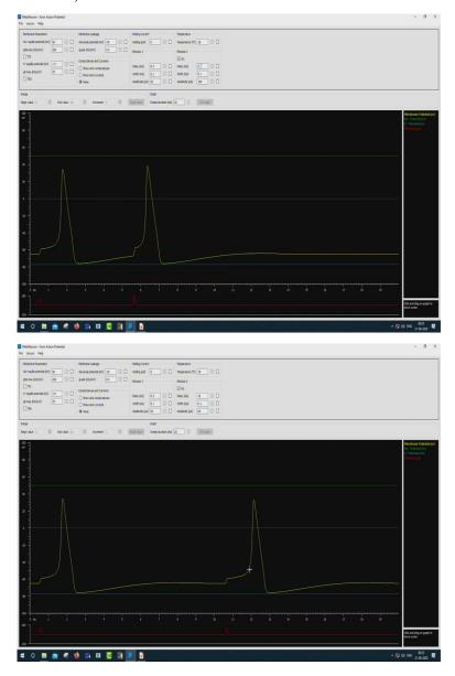
And after some time it will fire but you need a higher threshold, the amplitude needs to be higher and after about 10, it comes back to normal. So, with normal amplitude, it fires. Notice that when I change the amplitude from 100 to 65, it was slightly delayed so, the thresholds have changed.
