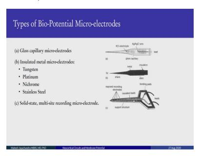
let us talk about the actual techniques, the microelectrodes which you need to record. The most used variety of electrodes are glass capillary microelectrodes. And here, you have a glass capillary tube, and one part is heated and pulled so that the tip becomes in the micron, 10-micron range.
