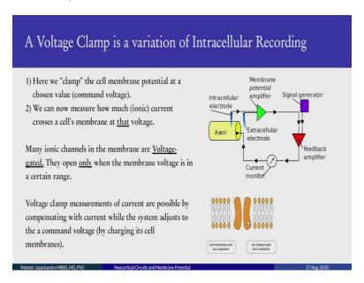
Further, they developed, Hodgkin and Huxley developed a voltage clamp technique which is a variation of the intracellular recording. Here we have the electrode inside, and we clamp the cell at a particular voltage, a command voltage it is called. And at that voltage, with the appropriate signal conditioning circuit, we record how much current crosses the membrane.
