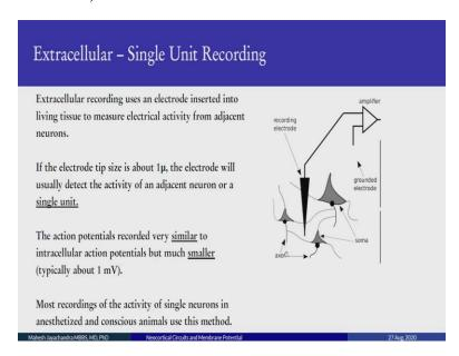
Let us consider extracellular recordings. As we had mentioned, here the electrode is very close to the neuronal tissue, it is not inside the neuronal tissue and it is just adjacent to it. If it is about  $1\mu m$ , 1 micron, the electrode tip, it would record the activity of an adjacent cell and that is called a spike or a single unit.
