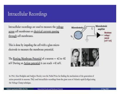
let us consider intracellular recordings. So typically, you have a cell, you have a microelectrode which we showed, a glass microelectrode that impales the cell, and then between inside and outside you record the potential. The microelectrode is connected through the silver-silver chloride wires to a microelectrode amplifier and then it goes to the signal conditioning circuits which either record the voltage of the currents.
