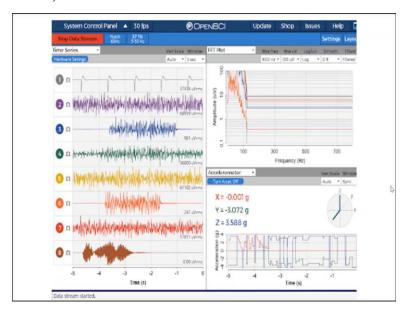
So, once you are open BCI Cytone or software is programmed and connected with wireless link and you start your data stream, the screen will look like this. This is for Cytone, it has a 8 channel as you can see here, you can select the notch filter and band pass filter settings from here, you can also see the FFT which frequencies are prominent in particular channel as well as this is an accelerometer, it shows the movement of your Cytone board.
