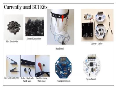
If I talk about modern day tools or modern-day components which have been used then we can see that currently used open BCI I just show you one open BCI get here. So, basically it will have a different electrode along with the leads to connect that electrode. Now, in the first image here whatever you can see is known as flat electrode.
