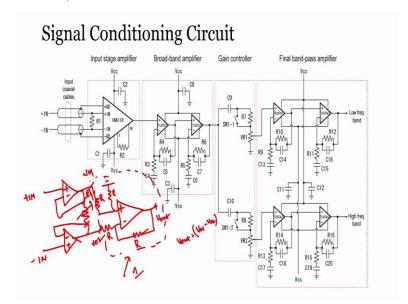
1, 2 a resistor in between, this is minus this is plus this is IN minus, this is IN plus. So, the negative terminal since we always require a negative feedback so this will be connected at this point whereas this will be connected at this point this act as gain, whereas it contains another operational amplifier, in differential amplifier configuration with a gain of 1.
