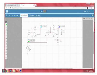
So, what I will do, go to the schematic, now we have to use the 3 op amp base instrumentation amplifier, since we do not have. So, here I will make it as instrumentation amplifier.
