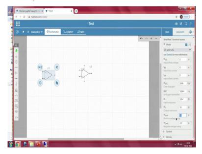
So, I will name it as test circuit, I will try to build an inverting amplifier. So, either you can go with three op amp based inverting amplifier or 5 terminal op amp base, the only difference between 3 terminal and 5 terminal is in case of 5 terminal it contains a external to other 2 terminals apart from 2 input and 1 output terminal.
