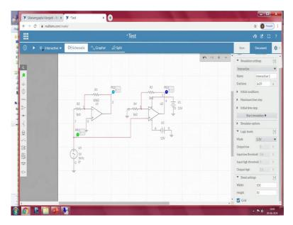
Here we can see the resistance, either we can change at this point or during the simulation industriously we can vary. So, in this case I am going with 1k and whereas I am changing to the 10k so the gain is 10. So, since is op amp is powered with plus or minus 15 the maximum voltage that you can see close to 14.3 something you can refer to the datasheet, it depends on the op amp that you are considering.
