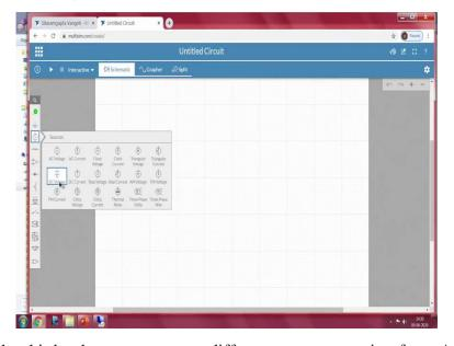
Similarly, on the third palette you can see different sources, starting form AC voltage, AC current, clock voltage, Clock current triangular wave DC voltage, so irrespective of, so if we want to perform any analysis using AC you can see any clock related you can apply any triangular voltages DC voltages everything is available at this particular toolbox or palette.
