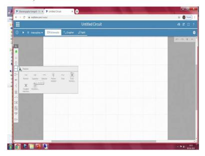
So, most of the our electronics circuit uses a passive elements like inductor capacitor and resistor, especially pots too. so all different passive elements are available at one particular tab passive tab where you can see all resistors, capacitors.
