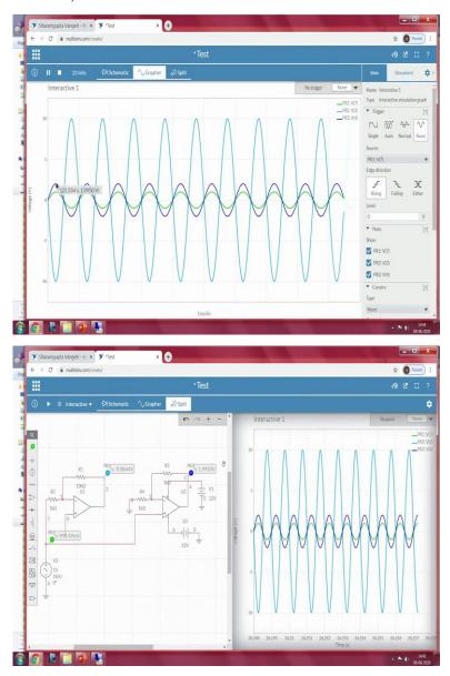
So, right now I am going with the interacting mode, whenever we go to the grapher we can see. So, we know the PR1 is input so the green colour represents the input which is 1 volt and PR2 is a output from the inverting amplifier configuration with a gain of 10. So, since the input is 1 the output is of 10.
