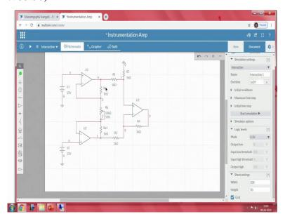
So, I will delete the previous circuit I need 3 op amps in this configuration I will take a 3 op amp base itself but 1, 2 but whereas this one I have to flip, two way of flipping it either we can go to the sitting and directly use it configuration pane or we can use the duplicate, we can use a mirroring and rotation method.
