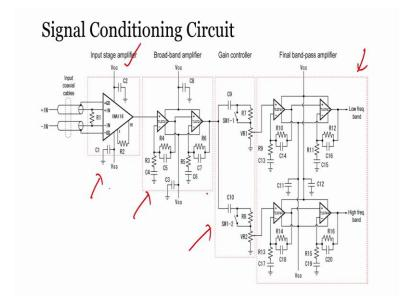
So, now when we come back to our slide. So, we finished about the input stage amplifier configuration the working of instrumentational amplifier we have also finished about we have also seen about a broad band amplifier and final pass amplifier and since we know about the gain controller part, so the idea of this gain controller is to act as a attenuator aware, it has been provided with SPSC switches two SPSC switches and R7 and VR1.
