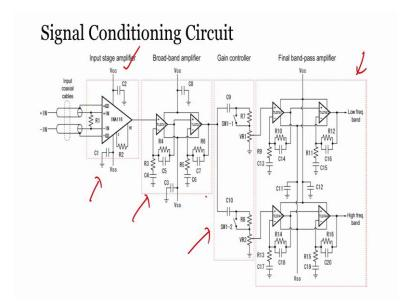
So, when we look into the gains of each stages when we consider input... based upon the design, based upon the resistor value that we have selected the targeted input stage amplifier is of 19.5 the target broad band amplifier stages of 93.5 and the attenuator third stage which act as an attenuator in this case is of factor of 9 and the final band pass filter is of 58.8.
