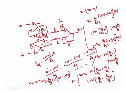
I will take the new page so that it will be easy to further discuss on this. I will construct an 3 terminal operational amplifier since we do not have INA116 in the online database of NA multisim. So, even it does not have an operation instrumentation amplifier configuration a 3 op amp base instrumentation amplifier I will show.
