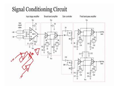
So, this is a signal conditioning circuit, so in the first stage, we have input stage amplifier where instrumentational amplifier, so now I will show you how to construct this instrumentational amplifier as we are all already discussed the use of instrumentation amplifier at this point and the use of INA116 and since we do not have the commercial we do not have the exact you know 116 in circuit simulation software.
