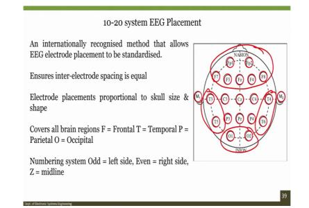
However, this particular class is more on understanding just a general concept about the EEG and the fabrication techniques for the same. So when you talk about EEG placement, you see this is the way they use, which is called 10-20 system for placing the EEG electrodes. And then you can see that, the numbering system on the system is odd for the left side and is even for the right side.
