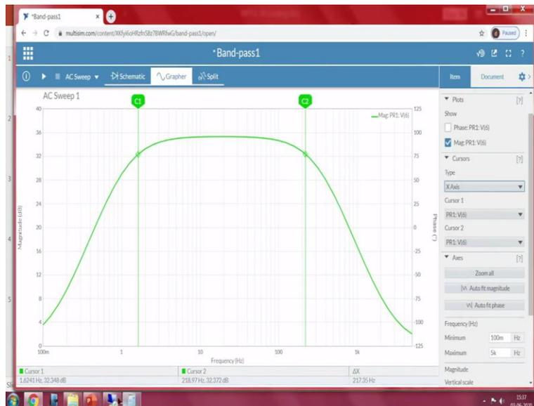
Similar to the previous one I will remove the phase part and I will go with vertical scale as decibel. So it is easy for us to understand what should be the 3 DB point. I will go with the Y axis. This is a top to the peak value and 3 DB is close to 32.351. So now I will change it to X axis 32.351. So, cursor 1 is almost close to that and cursor 2 will also get to the same. So, now here we can see, we got somewhere around 1.62 hertz to 218, 281 hertz.
