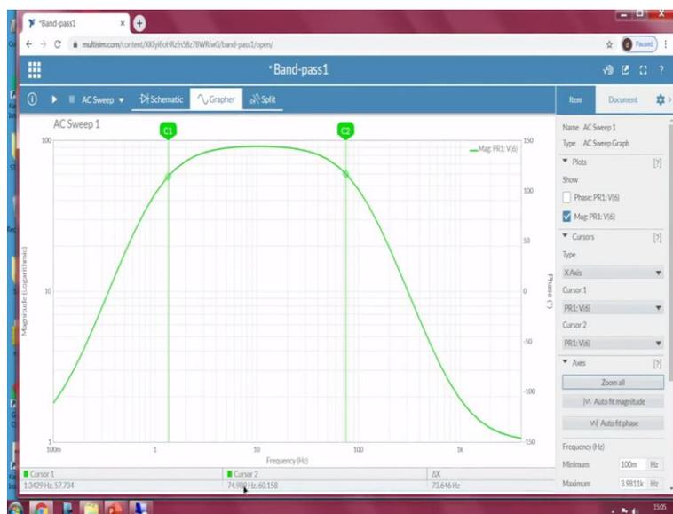
So, this particular plot is an indication of the magnitude at the output of the second operational amplifier, whereas, the dotted line dotted green line is an indication of the phase here we can see. So, further, since our understanding is to find out the cutoff frequencies, upper cutoff and lower cutoff frequencies of the design the filter what I will do, I will disable the phase part-time be I
