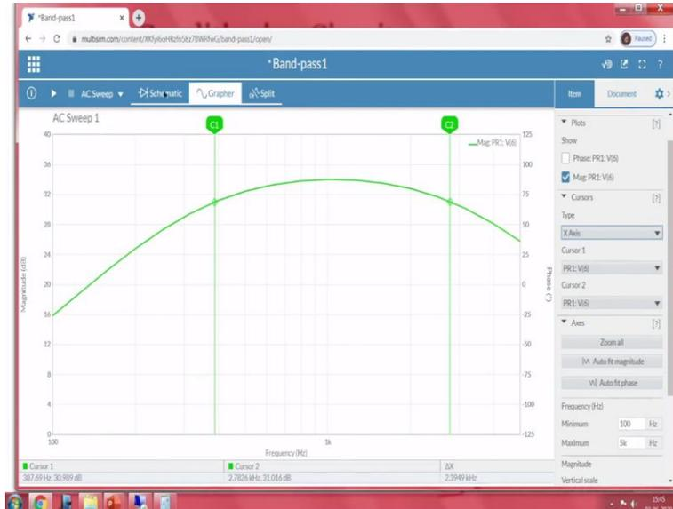
Simulating it yes, phase switching off then B then let me put Y axis cuts so that we can analyze DB. So, instead of changing to logarithmic, I am going to decibel point. So, here and minus 3 DB somewhere around close to 31 31 DB. So, now I am changing it to X axis 31 DB. So, here we can see the this particular circuit can pass frequencies between 387 hertz to 2.7 kilohertz whereas target is 320 hertz to 3.4 kilohertz. So, with this, we can understand the implementation
