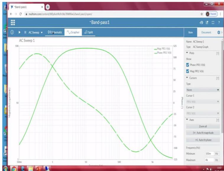
So, when you go to the grapher, here we can see that the thick green color indicates the magnitude of plot of PR1 V6. So, PR1 V6 is nothing but this 1. So, V6 is nothing but voltage node 6. PR1 is probe 1, the intention of probe 1.
