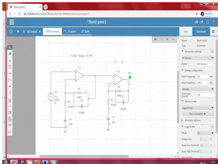
Final stage of band pass filter when we see the AC sweep analysis.
