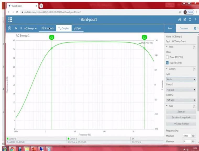
2 3 4 5, so I will change the phase, remove the phase, and go with my magnitude. So, I changed the settings as 10k. Now we can see the plot from 100 milli to 10 k hertz. So similar the same way at 3 DB line 1 2, somewhere close to here, similarly even at this point 1 2 3. So, we can see, we can achieve 1.3 hertz and 2.92. So, we can add to the close to what we have targeted for, but
