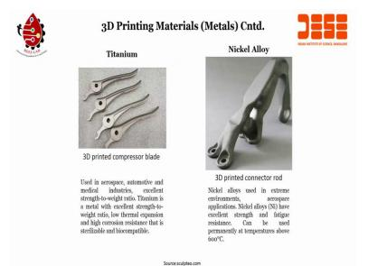
Titanium and nickel alloy. Titanium is used for a long time, is used in medical industries, it can be used for implants, it carries an excellent high strength-to-weight ratio, is low thermal expansion, high corrosion resistance and it is biocompatible. So, generally, the blades are used or the implants are used, are made up of titanium.
