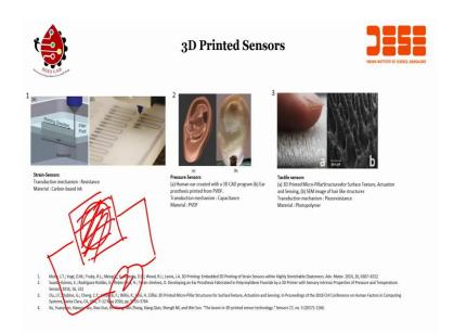
But the real application of 3D printing will be in sensors, will also be in casing the electronic modules. And you can here see that we can directly use 3D printing for fabricating sensors. For example, if you want to print carbon, carbon-based ink then you can create a resistor. For example, if I move my 3D printer such as I can print the carbon, carbon ink then what I have?
