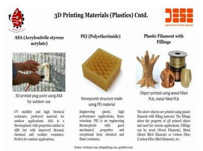
So, like I said you can, the choice of material depends on the application. Fewer materials are there which are ASA PEI and plastic. Where the plastic filament with filings or fillings are used for, for several applications like you want to fill, can be wood, metal, filament, or carbon fiber. Where if you want to use PEI, you can use it for honeycomb structure, this is just an example.
