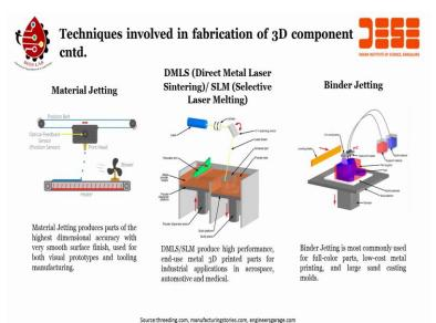
So, if you see the slide we have three different techniques. Material Jetting, Binder Jetting, and Direct Metal Laser Sintering. So, in Material Jetting, the Material Jetting produced parts of highest dimensional accuracy and you can see here there is a blower which will blow and, and dry the material. There is a heater on which the, the material is printed using the printed head.
