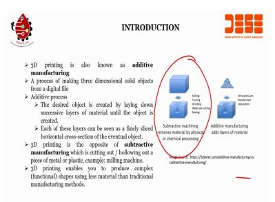
So, let us see what exactly 3D printing is and we will take it over. If you see the slide, 3D printing is also known as the additive manufacturing process. Why additive? Because it will add the layers to the substrate. While there is another machining technique called the subtractive machining technique. Where the material is removed by physical or chemical processing.
