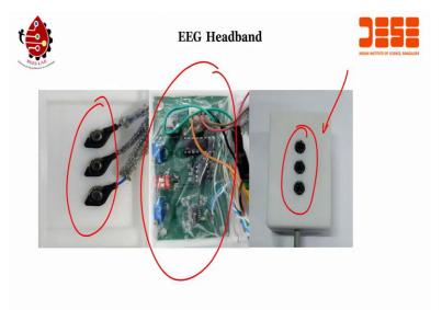
The application as, as I was talking about, you these are the EEG electrodes, recording electrodes. And this is the electronics that are used to process the EEG data. Now you want to cover everything in one box, then you can print this particular 3D printed casing, and you can cover it. With these 3 electrodes, you can place it on the scalp to record the EEG signal.
