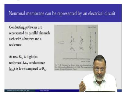
So, the conducting pathways besides the capacitance they are represented by parallel channels because in the membrane with the phospholipids membrane, you have sodium channels, you have potassium channels, so each of these channels has a battery and a resistance, the battery is the electromotive force which pushes the ion into or outside the cell.
