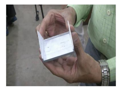
Now, bending is over without using height gauge or measuring tools and then we see that with that development drawing itself we have made the piece. Now, we have to make a cover for this one which we have to measure this one and then I make one more development drawing and then test it and then the same similar way thing can be done.
