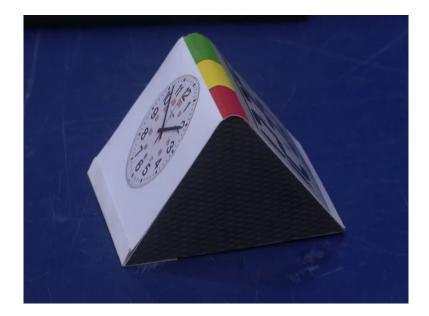
My name is Singh. I would like to demonstrate the sheetmetal fabrication of this timer without using height gauge or measuring tools. What I am doing here is I will take a drawing scale one is to one of a development drawing and then paste it on the sheet metal.
