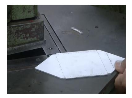
So, now the 4 sides of notching has been done. Now, for bending the limb actually we have to give a relief there are the 4 sides we have to give relief there. So, that it bits inside when we bend the sides. So, it will be plane there.
