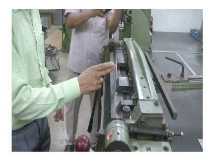
Now, we see that that is the bending line the dotted line. This is the folding machine where we have to adjust for various thicknesses adjustment has been made. Now, we have to keep the dotted line straight on to the fingers and then bend it. We can see that this is exactly 90 degrees bend. We can even measure this one.
