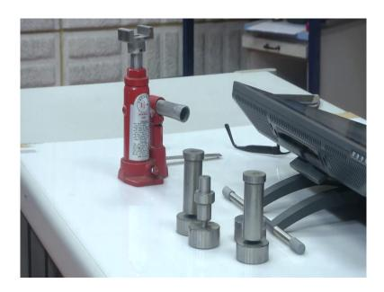
In this case of materials this is probably I meant for a softer or aluminium materials which we stock. In this the clearance is actually only 100 microns, which it is like taking the difference between a paper shear, difference between a cloth shear and difference between a tin shear. Tin shears and all have a different clearance and that blade angle compared to a paper shear and I think you know about it hobbiesh hobbing scissors how they do and so on like that.
