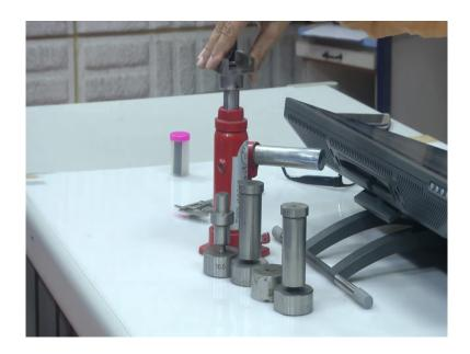
Then another important thing is which was required for us is saying; I completely miss the requirement for a small grub screw there, that grub screw has multiple things. One of them is it will prevent this from coming off. There is a small change in dimensions here; so if I tighten the grub screw, it will see that it cannot come out easily. Secondly, even see, now it does not come out, this orientation also depending on the way we want easily we can fix the orientation.
