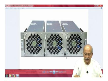
I am not sure what it is. I expect that it is either a dummy load or it is a some other power supply which is remotely addressed and controlled. Three of them are mounted in a possibly what looks like a 3U sub rack. Seen that again mounting holes and something here you come to a very very important things. Heavy items cannot be directly mounted with the flanges, so, end up with a tray instead.
