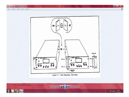
This is taken from a just around what you call 40s 50s, possibly in the 50s when this people where the standard equipment to be mounted into a rack. So, add a pressure here and take the front panel add a adapter plate here, adapter plate here and then join this two and then we can have a rack mounted 2 units on one thing.
