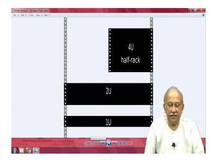
So, all the stacking eventually lead to what is called the rack system. Rack is not the one that is used know. Where enforcing your political correctness it was used a rack means anything which is vertical and another thing is it has regularly pitched openings here.
