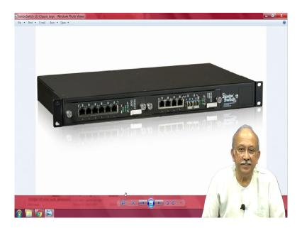
When you make such equipment, you probably have usually 1U that is 44 millimeters available and the full width of external is 482, inside up to 450 mm back is 450 m. So, typically safely you can take 440 mm, where you need to use; seen that what determines the front panels what determines. This now another detail, it may be useful for you here. Notice something here, there are again two screws or I will call it some thumb (Refer Time: 22:21).
