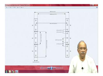
So, in the course of building systems this so called 19 inch rack came about. You see here, you will see 19 inch and the 19 inch they refers to total width of the support structure. And in this case two things which are important one is you have mounting openings and the other is the extreme width of the front panel. So, if we go back here you will notice that this represents a height and this two represent the mounting openings. Now, we wanted relatively universal.
