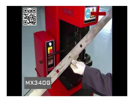
So, in the case of regular production what is done is things are made repetitive by using proper jigs and fixtures. One of them in this case is a simple stopper, to maintain pitch, it is fed to the stop. In the process sheet it is read know, using fed to stop. After it is fed to the stop the punch is operated, so you can see here next operation progression takes place, next operation takes place.
