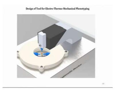
In the video what you have seen, you have seen that there are indenters and in the indenters, there are the blue color thing which is indenters at the tip of the indenter we have attached the chip that we have I have just shown it to you. And, these chips are used for understanding the electrical and thermal properties while the top indenter it presses tissue from the top.
