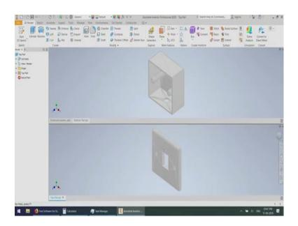
So, we will be using this bottom part file and the top part file for 3D printing. So, I will select this bottom part, and then I have to save this file for 3D printing. So, this Autodesk inventor software I am using is saving the parts in a dot it formats I want some other format that can be readable in the 3D printer software.
