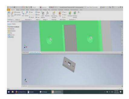
Here we can see these two holes are aligning. Here there is a little bit different because this circle diameter is 3 mm, and here this is only 2.5 mm. Similarly, on this circle also this hole also.
