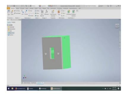
I will click on the constraint here; it is in the mate option I will click on the surface, and then found the surface; I click ok. Here see how our enclosure is ready. So, this is just looking like a square enclosure. So, for good aesthetics, we can give a fillet to these edges that mean, we can make these edges a little bit curvy. For that, before doing that I will save this file.
