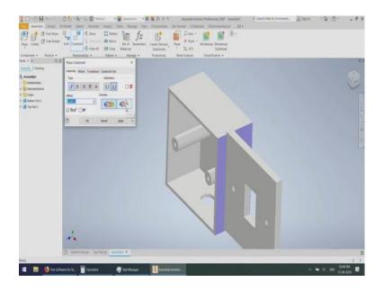
Now, I jump to the mate option I will click here in the flush option. Now, this is the way I wanted, but the top part came inside the bottom part, it is ok. I can move. Now, I want to constrain this surface and this surface in the same flush joint, I click ok. Now, I want this small surface and this surface to be in touch with each other.
