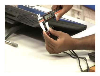
Today I will show you how to make an enclosure for a switch. Is a symbol switch, inside there is a light. first I want to measure the dimensions of the switch to make an enclosure. for that I will be using vernier calipers, this is a digital vernier caliper.
