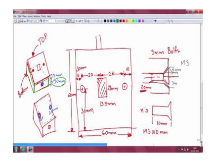
And we will be making an enclosure. suppose this is the enclosure, the top view of the enclosure here the switch will be, the switch will come. And we can take the connections through here on the side. And we can give two screws here and here. for designing that, we have to fix a dimension before going to use the CAD software that will be easy for designing. this will be 13.5 mm and this will be 21 mm, and we can use 2 bolts to screw the enclosure.
