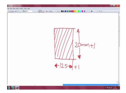
As we measured, we have a switch; the switch has a height of 20 mm and a width of 12.5 mm. this is the exact dimension of that switch. for making an enclosure, we need a hole which is greater than this dimension, this dimension 20 mm and this dimension 12.5 mm. Otherwise, the hole in the enclosure we are making and the switch dimension will be the same.
