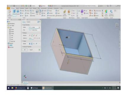
Now, we can only see a rectangle we do not know it is a 3D object or not. for viewing this as a 3D object, we have to rotate this object. For easy rotation, one option is we can use this option we can click here and drag it. Now, here we can see this is the 3D object. There is another shortcut for rotating, we can hold the shift key and hold the scroll button and we can rotate like this.
