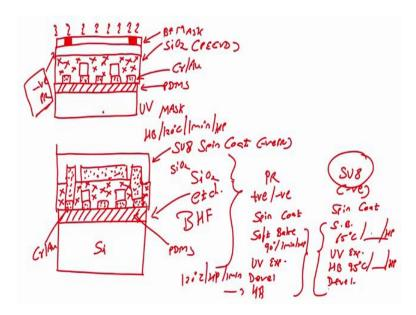
When photoresist gets stripped off, my wafer that I have a pattern like this looks similar to my pattern number VI and this particular platform, what we had done We had a substrate with PDMS and PEDOT PSS a strain gauge on which we have insulating material which is step number V, and then we have performed of photolithography and remove the contact; then we are deposited chrome gold and we have patterned to form the gold pads.
