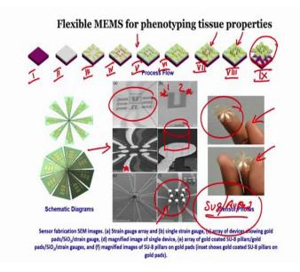
if we see the slide what we are seeing is, the step I where we take oxidized silicon substrate; step II where we have spin-coated PDMS, step III where we have the form of the pattern of chrome and gold, and step IV where we have formed the piezo resistor. these are an array of piezo resistors, 18 numbers; this is a single piezo resistor SEM image of that.
