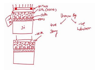
But if I deposit gold directly on this then it will get short; that is the next step would be, I will deposit insulating material and this insulating material the pattern would be this x cross ok, this is my insulating material. if I have this one, then what I will do is; I will spin coat photoresist resist and this time I will spin coat negative photoresist, then I will load the mask.
