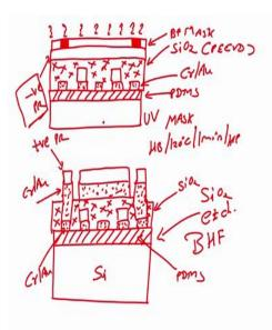
The next step is I will dip this wafer in the gold etchant, then rinse it then I will dip. after this of course; there is a hard bake, 120 degrees 1 minute per plate followed by dipping the wafer in the gold etchant, then rinsing the wafer, then leaving the wafer in chrome etchant, rinsing the wafer.
