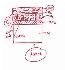
The area which is not exposed will become stronger; the area which is exposed will become weaker. Now, can see that we have positive photoresist, we have positive photoresist and here we have open the window; there is a window that we have open correct. Now what we will do know, we will deposit gold or a metal everywhere, chrome gold, asr chrome gold everywhere and then the next step is we will dip this wafer in acetone.
