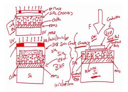
now we will have a mask, we know that SU 8 x is a negative photoresist and we want to protect SU 8 in the center. what we will do We will use a b field mask and by using the b-field mask what we are doing; we are protecting the layer of SU 8 which we do not want to get develop in the SU 8 developer.
