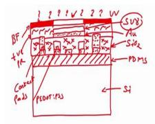
let us see here on the slide. have this particular thing. I will draw it, here again, it becomes easier and we will start from there. again I am repeating please focus here, have silicon substrate, have PDMS on silicon substrate al. This is r PDMS, this one is r silicon, then we have in, we have contact pads or contact electrodes. Then we have here PEDOT PSS strain gauge, then we have insulating material which is by silicon dioxide, al.
