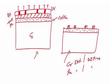
Simple, see take a glass slide glass; then on that, coat metal, which is r chrome gold, then spin coat photoresist, positive photoresist, then use the mask, b field mask, something like I am just showing a representative diagram al, b field mask.
