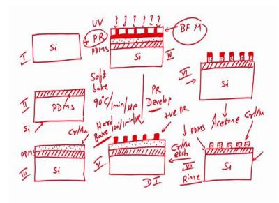
I will show the process flow in detail. The first step is take this silicon substrate, silicon; the second step is to spin coat PDMS on a silicon substrate. let us say this is r PDMS ; then the third step is to deposit. this one is PDMS, this one is still silicon, this substrate is still silicon; the third step is to deposit chrome gold on PDMS. let us say we have now silicon, we have PDMS and this one will be r chrome gold, .
