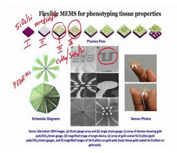
We have taken a silicon substrate; we can take an oxidized silicon substrate, on which we have spin-coated PDMS. Silicon or silicon oxidized silicon then we have PDMS on the silicon, ; this one which is step number III is r chrome gold pattern on silicon dioxide or oxidized silicon substrate, .
