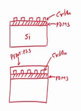
if see the slide, have this particular substrate ready with r gold pattern on the PDMS, is not it; silicon, this one would be PDMS and then have r gold patterned in this way, is not it. now, what we will be doing in the next step is; the next step we will spin coat, we will spin coat P dot PSS on to this chrome gold or on the wafer, which has PDMS, this is P dot PSS . After this, the remaining steps are exactly similar to these slides, see I will show it to .
