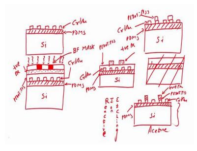
if I take a cross-section of this particular piezo resistor which is made out of a P dot PSS, then for that the mask that I am showing here will look like this and this is a b field mask . A photoresist is a positive photoresist and mask is a b field mask, . The next step would be exposed to UV light.
