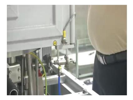
And metal piece you are seeing is grounding; is grounding between the is the door of the chamber, is the chamber's main body those two are grounded. as to protect the user; so those things are there. cable you see let me let us focus there.
