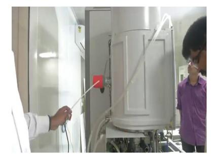
just now I have shown you the Pirani gauge; the angle valve, the high vacuum valve, the turbo molecular pump inside. I told you we have seen the penning gauge, but I am not sure whether we saw it yesterday. here you can see the penning gauge here.
