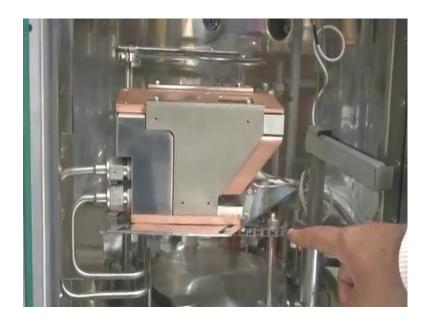
We have seen the substrate holder rotation before, now we will see the source rotation. We can see the crucible holder now we are changing the speed of the rotation here we are changing the source. you can see the belt here moving changes the crucible. you can see the belt moving; now let us look at the crucible, we will go inside and look at the crucible moving.
