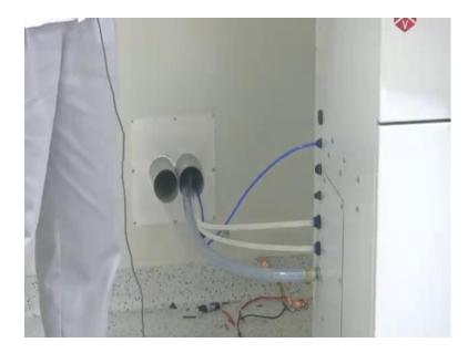
These two are processing gasses; the other two are for the purging and the creating vacuum venting for general gasses we are are used like nitrogen compressed air and all. those connections are made. we are ready a bit to show you exactly the functioning of the control panel, how vacuum is getting created inside the chamber and for the E beam gun are we getting the plasma all those things. once it starts we will see .
