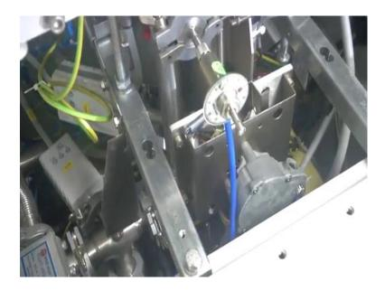
is the high vacuum valve for the connecting chamber.
