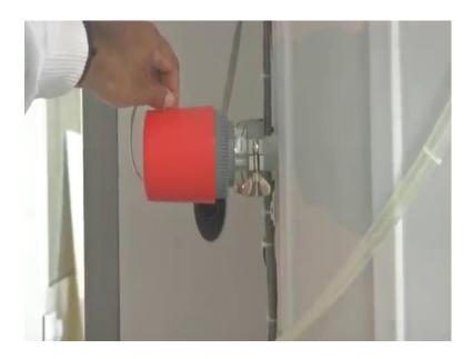
It is called the cold cathode gauge also. the data for let what is the pressure it is measuring comes out through Ethernet cable is connected to here. is the gauge is connected to the chamber here in the chamber is very very cold because of them; so line you are seeing here on the chamber has a cold water circulation inside is for cooling the chamber; so is there.
