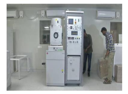
Now, we have finally, pushed the power supply into the control panel housing. Now, we will make the connections from behind. We have made three-phase connections with a good ampere rating for this power supply unit. And this power supply unit will power the control panel, separately on the left side you can see the chamber. The chamber will have its own separate power supply that will be supplied through a dedicated connection.
