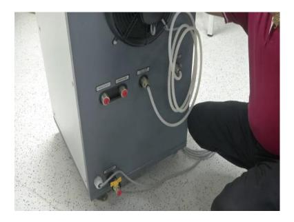
After water contamination can drain the water from through this valve, drain valve. Clean the tank water, tank and refill fresh water.
