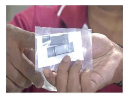
So these are the crucibles where if we keep the material it can be (Refer Time: 32:39) deposit. So, this is tungsten crucible. So, why we have different materials, is depending
