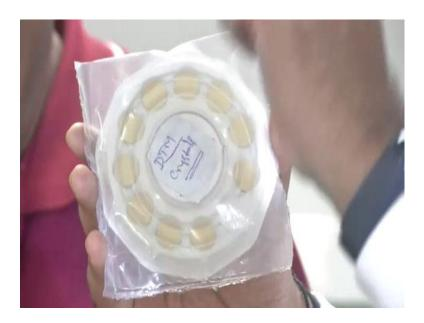
These are crystals, so you can as we have seen inside there is a quartz crystal molybdenum inside, that is very critical because that measures the deposition rate and the thickness that is deposited. So, the thing is the crystal also makes deposited not in the process.
