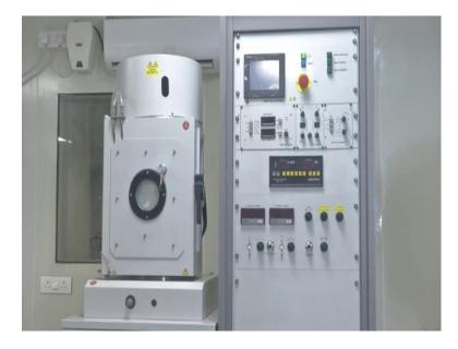
Actually, first switch on the water pump wait until this 5 to minus 2 in the (Refer Time: 13:21), switch on turbo. For switching on turbo need water also, without water it is not getting run.
