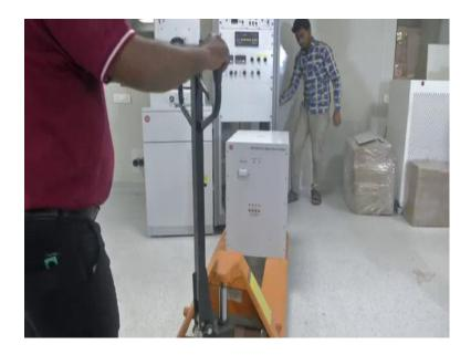
Now, as you can see we are pushing the power supply unit for the electron beam, electron beam power supply into the system into the housing of the system.
