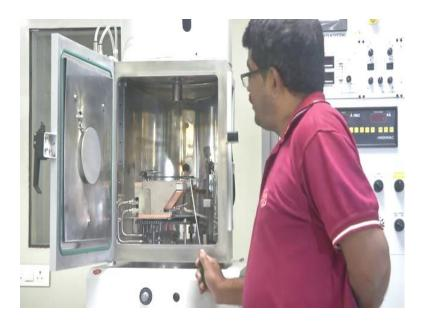
EB gun, electronic beam gun. Here we have EB gun shutter, this is a pneumatic shutter, this is a LT, this is therma (Refer Time: 20:30) shutter, like filament, boat or basket.
