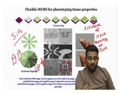
These are the gold pads 1 2 3 4 5 6 7 8 and I zoom one gold pad what do I find, I find that the gold pad looks like this. Why? Because, below gold pad there is an insulating material; wWhat is that insulating material? Insulating material is my silicon dioxide . So, silicon dioxide is used as an insulating material and we have a strain gauge on the bottom. So, it is like of strain gauge insulating material on that you have the gold pads, this guy .
