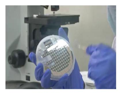
Now, we have I will show you the substrate that has been patterned through liftoff technique and diced as well. So, diced using wafer dicing machine, so that way because you will not be seeing the devices in a full silicon wafer, but it is a diced silicon wafer. So, you can see it under microscope so under the camera. So, this is this is part of a whole silicon wafer ok, but what we did these are individual chips you can see, we have diced this wafer.
