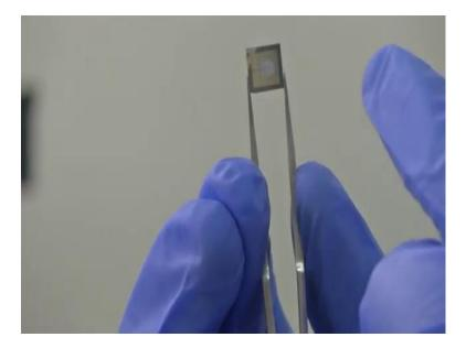
You can see the sensor in my hand here. You can see a bright spot a white color spot at the center right that is because it has been coated with an active material for sensing applications, and underneath this active material you have electrodes.
