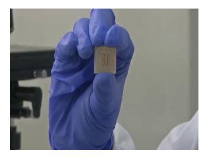
So, in my hand let us look at it in close. In my hand, I have the sensors which you can see and their contacts have been wire bonded on to these pads and these pads can be taken from here. So, now, it is very easy to solder onto it this is like a PCB this is a PCB only from the sensor we have wire bonded onto the PCB and we can take out from the PCB. See this is part of packaging, it is called MEMS packaging.
