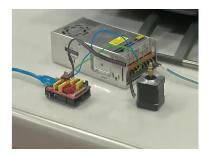
So, you can see here; you can see the stepper motor over here correct this is the NEMA 17 stepper motor and I have got an SMPS here this stepper motor requires 12 volt power supply for it to work. So, I connected a SMPS that can provide an output of 12 volt and it goes to a board over here this is an arduino uno board on the bottom and this is a CNC shield.
