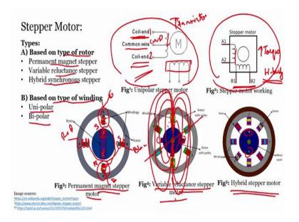
So, there are different types of stepper motor and we classify them based on type of the rotor based on the type of the rotor we can classify them as, permanent magnet stepper motor, variable reluctance stepper and hybrid synchronous stepper ok. So, you can what you can see here is, this is the permanent magnet stepper motor, now I will tell you the concept of how it works ok.
