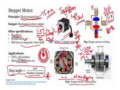
So, this is a different kind of motor as you can see on the presentation. So, stepper motor is a different motor like our DC motor only, you can see a say stepper motor a type of stepper motor named as NEMA 17 stepper motor over here ok, you can see this black part with a black part is the body and this is the shaft that rotates ok.
