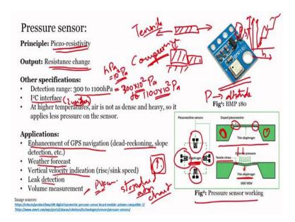
So, now I will be showing a practical example of pressure sensor like that. So, today we will be discussing about this BMP 180 sensor that you can see on this side ok. So, this is the pressure sensor that we are going to discuss today ok. So, BMPs like many other sensors that are working based on piezo resistivity. So, you must have also heard about piezo resistivity piezoelectric nature and so on.
