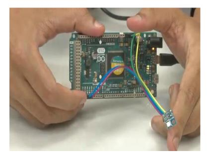
So, you have here the casing with the thin diaphragm inside and four cables come out of this out of which one is 5 volt one is ground and then there is SDA and SDA and SCL ok. These are the two connections that we use for I square C communication you can see here I have already connected it ok. Now we will move on to the arduino programming ok.
