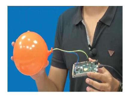
So, I have put the pressure sensor inside the balloon ok. So, it is like this now you can see that the pressure sensor is within this and I have connected everything. So, theoretically what should happen is when I compress this the volume decreases and the pressure should increase, but since this is a balloon can deform it can deform. So, if the pressure in change would not be so visible, but still you can see a pressure change in the serial monitor ok.
