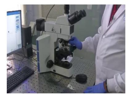
So, this is a metallurgical microscope. We have x, we have see seen about this microscope and all in the part of this course. So, I have kept the sample here under 10 x magnification ok.
