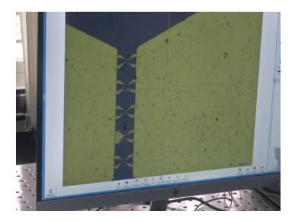
I am at 50 x magnification and I am adjusting the focus. Now, you can see the interdigitated electrode structure here. These are the main electrodes; you can see the interdigitated electrode structure at 50 x magnification. Very delicately, we have to move the substrate. So, you can see the electrode structure. I can even go to 100 x magnifications and show you. I am going to 100 x magnification now.
