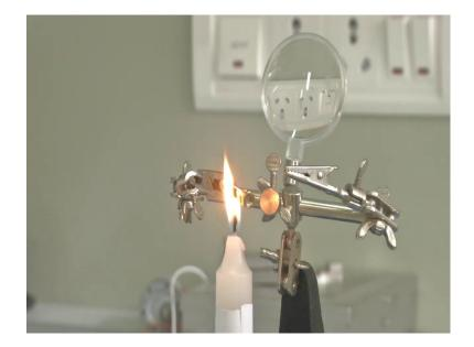
Now, let us see how the temperature induced phase transformation using SMA can be performed using Joule heating; that is nothing, but the actuators are typically actuated electrically by Joule heating. So, the entire mechanism of training will be shown to you with me here is Rabeeh, who will show you how to train shape memory alloy. So, what he has here; to initially you have to fix the SMA into the shape what you require, and then you have to heat it.
