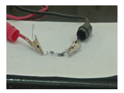
So, here we have removed it, once we have heated it up to 400 degree Celsius, next what we do is, we have it here; the SMA is removed from the test bench or the table where we had you initially just heated it. And after uncoiling, we have connected to the supply. So, slowly just like sub give some 2 volts and then 0.5 Amps slowly increase current.
