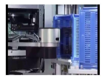
A robot scans the wafers and determines their quantity, position and size and the processing begins.
