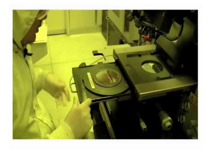
So, again you press load and it says pull slide and load substrate onto chuck.
