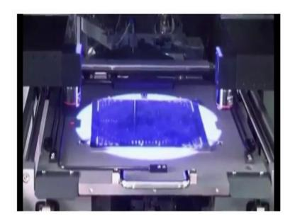
The microscopes only move sideways, thus reducing the vibrations of the alignment stage to a minimum resulting in far greater accuracy.
