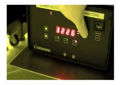
So, you know that the light bulb is on but in addition to that you want to find out how many hours are left on the light bulb. So, you check the power supply. You hold this button called DS. It says 3226; it is how many hours the bulbs being used. So, the bulb has a lifespan of 4000 hours. So, when it is over 3500 we would notify staff and tell them
