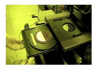
We press this button where it says load wafer. So, it says pull side and substrate onto chuck. We will just load the wafer on and when it is in, you press enter and it will bring it up.
