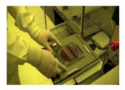
So, would you load your mask in here by lift, lifting this clip here and putting it in and when it is in nice, you hit this button called enter; you can toggle the vacuum. So, right now the vacuum is off. Then you press enter now the vacuum is on when you come back you can see that it is it is vacuumed in and is stuck pretty well. So, now, we are going to put this in here.
