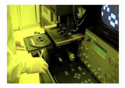
So, you press expose and when you do exposure again. So, then you turn away so the UV light does not a choice. So, after your double exposure you would unload your wafer. So, it tells you pull slide or unload substrate. So, you pull it out and then you take
