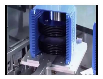
The MA200 compact processes wafers and substrates up to 200 millimeters regardless of their material, size, shape and thickness. The machine runs and adjusts fully automatically.
