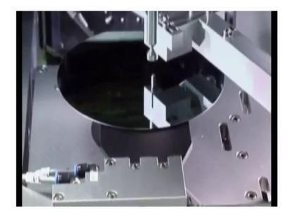
A linear transport system loads the wafer onto the exposure chuck which together with the robot arm guarantees the optimal and the flexible handling of the substrate.
