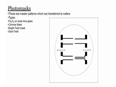
Hi, welcome to this particular module. We talked about photomask right pause bright field photomask and a dark field mask. So, this mask are master patterns which are transferred to wafers and the types of photomask are the Fe 2 O 3 on soda lime glass. It can be a chrome mask, it can be bright field and dark field as you know.
