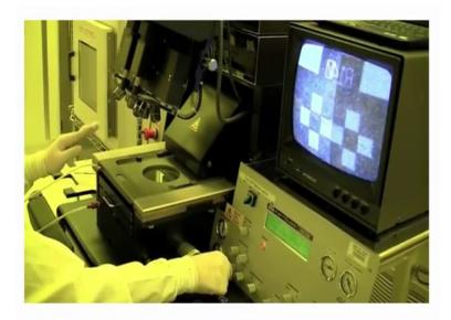
Now, we make sure this thing says backside alignment microscope is on. So, it is on, but also, we need to change this to backside alignments. So, it can be either top side alignment or it can be a backside alignment. So, this is an illumination. So, now, the light is coming from the backside.
