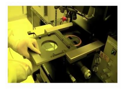
So, we carefully carry it. We will place it all the way in and when it is in, we press change a mask and that is how you load your mask. We are going to be doing a backside alignment now. So, what this does is it aligns features on the back of your wafer to your mask and how you do it is a microscope from the bottom. So, the first thing we do is we have to have a mask loaded and then we turn the screen on.
