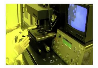
Then you press enter when you did that, and the microscope will automatically come down because we have the BSA microscope light button off. So, now, it is down we turn the TV screen on and what this is doing is taking it, putting the image from here onto the screen.
