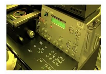
So, we just turn it to the ON switch. Now, you can see the machine starting up and it is important to read the screen, it tells you a lot of information. So, it says ready for start, press load button. So, the load button is right here. Now, we press that and now it says watch out machine is starting load.
