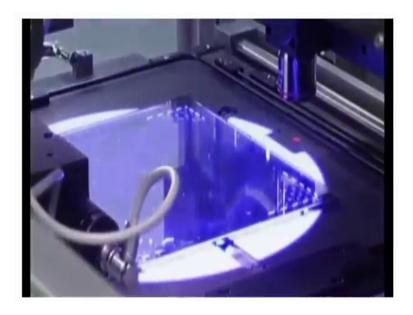
The big advantage over steppers is the exposure of the entire wafer in one step.
