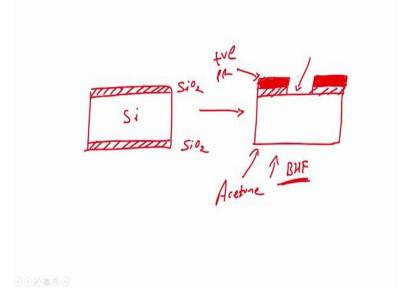
So, once I perform photolithography; what I will do here, is at I will create a window into silicon dioxide and then I will etch the silicon through that window.
