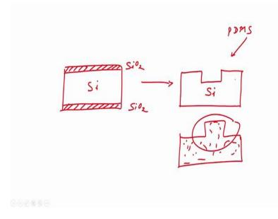
So, we have a mould, on which if I spin coat or if I pour PDMS, this is my PDMS and cure it; after curing I can strip it off, what will I have? I will have PDMS structure like this, right. So, after I strip it off, I can get back my mould; and I have already patterned my PDMS using this particular silicon mould.
