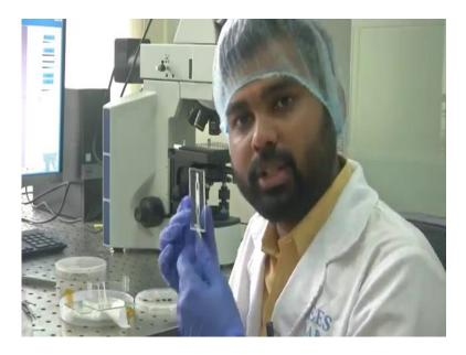
But these are mass produced microfluidic chip, these are all, these are also we have made in our lab. These are mass produced microfluidic chips; but because these are mass produced, they do not employee, they complex micro fabrication techniques, instead we use very fine laser cutting.
