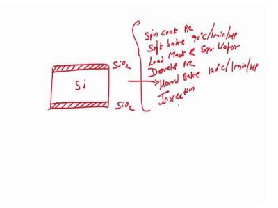
So, if you see the screen the, if I have silicon wafer right and if I grow silicon dioxide; let us say I am growing 1 micron of silicon dioxide.
