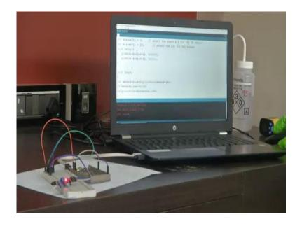
So, in the arduino code, you can see that I have define the sensor pin as three; that means, the digital output of the IR sensor have been connected to the pin number 3 and the buzzer is connected to pin number 22. And, in the setup I have define the buzzer pin as output means the buzzer is going to give an output that is the sound beep sound. And the sensor pin is the input, and I have defined it because the sensor pin is connected to a digital input pin that is pin number 3 ok.
