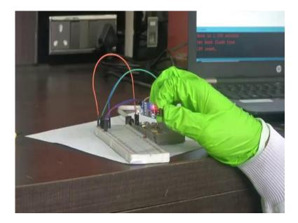
So, this shows that the IR can only be used when it comes to a obstacle or an object that is white or have a reflecting surface ok. So, this is about the IR sensor.
