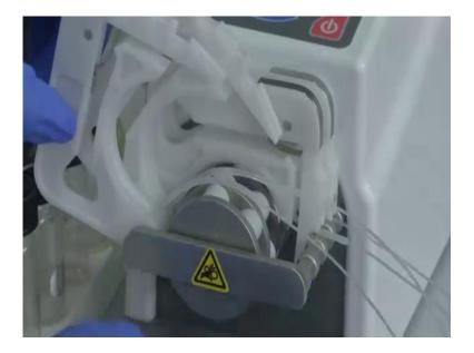
Here there is like I mentioned these are called as the cassette and when we remove this cassette this is the tubing bed 1, 2, 3 here like I mentioned in the previous case there were 3 rollers; however, here there are 6. So, the number of rollers can vary from 2, to 16 depending on the number of pulses which can be generated as your fluid flows that is a pulsating flow of the fluid.
