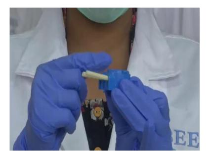
This these are again called as silicone tubings through which the fluid can be pumped.
