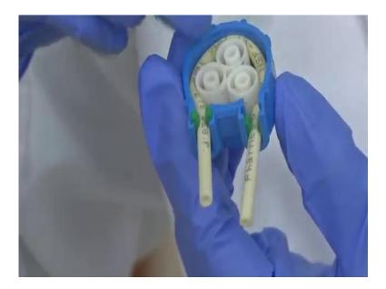
And here what we see is nothing, but these are the rollers 1, 2 and 3 rollers. So, what happens is as the motor drives it pushes the 3 rollers at the set R P M. The RPM in which your motor is driving it drives the 3 rollers here and the surface here the tubing which is here in between the roller and the outer casing if you observe is compressed. So, what happens is as it moves
