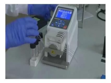
Here as you can see this is a peristaltic pump a tabletop pump with 4 channels 1, 2, 3 and 4 when we have this device. So, it has one inlet and one outlet and when we do a comparative study the dimensions of this silicon tubing is much larger when compared to silicon tubing which is here. So, this has 1, 2, 3 and 4 channels and you can program it to have a different r p m depending on the requirement.
