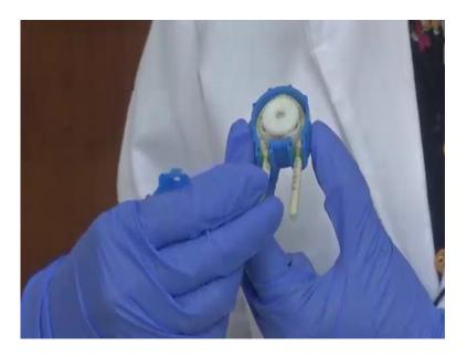
So, when we remove the casing from bottom these are the tubings.
