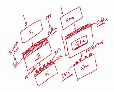
So, what should I do, for if I want to make the device on silicon wafer, I have to first grow silicon dioxide. This is SiO 2 what is SiO 2? SiO 2 is your glass. On this SiO 2, I can deposit a metal and I can do a lithography. I can perform a photolithography, alright. So, this is my interdigitated electrodes, this is my silicon dioxide, and this is silicon wafer you got it.
