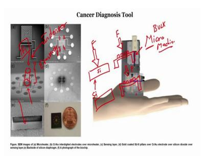
So, we need to create this diaphragm. We have to etch the silicon wafer to create the diaphragm. How to etch the silicon wafer? There are there is a technique called micro
