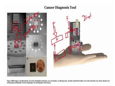
So, suppose I have a silicon wafer and I have a silicon wafer with a diaphragm, like this. If I apply a force here and I apply a force here which one will bend, this is not going to bend because silicon is solid material hard material this will bend. So, here what I will see, what I what we are expecting is? It will bend like this; in this case nothing will happen.
