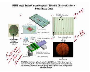
So, if you see the screen, these are the interdigitated electrodes here and what will be the impedance of this? Impedance of this would be infinite or extremely high, why? Because there is nothing on this interdigitated electrodes and only there are metal lines not connecting with each other. You see here there are metal lines not connecting with each other; these are lines which are not connecting with each other, correct.
