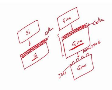
In case of silicon, let me draw little bit smaller schematic, silicon. Can I deposit a metal directly on silicon? This is my chrome gold on silicon wafer. My question is, in case of glass, I could directly deposit chrome gold on glass and pattern it to form interdigitated electrodes. In case of silicon, can I do the same thing? I cannot, why because glass is an insulator while silicon is a semiconductor.
