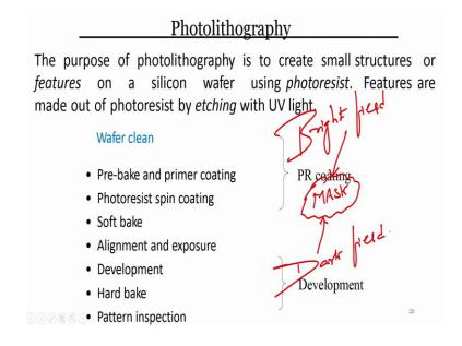
And when we talk about mask masks are two types of bright field and dark field; bright field and dark field mask . this is about your alignment and exposure. After that, you have to develop the wafer.
