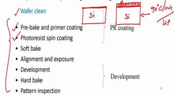
So, I will take a wafer, I am drawing a cross-section of it right, let us say it is a silicon wafer then I clean the wafer. After a free cleaning, I will heat the wafer or pre-bake the wafer at  $120^{\circ}$  C and then I will coat primer. this is a like a primer coating, a thin layer of primer is coated onto this wafer. This will improve the addition of photoresist. After the primer coating, the next step is, primer coating, next step is photoresist spin coating.
