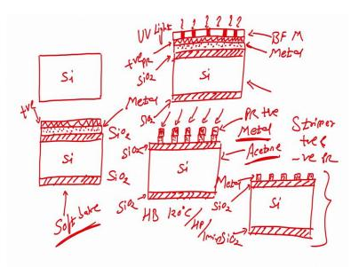
I have a silicon substrate, I want to deposit metal. If I want to deposit metal, I will have an insulating layer because silicon is a semiconductor. I will grow let us say silicon dioxide Si O 2, this front and back. Next step is I will deposit a metal. the dotted pattern is of metal.
