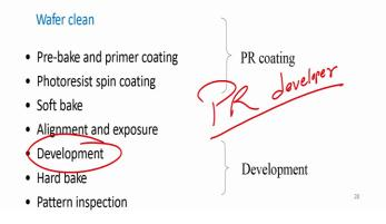
Developing wafer can be done with the help of photoresist developer. After you develop photoresist, the next step is hard bake.
