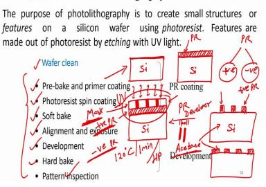
So, I will expose this with UV light. After I expose it, I will unload the mask and dip this wafer in a photoresist developer. When I do that, what will happen? That if it is a positive photoresist, if a positive photoresist, I told you photoresist are two types, positive and negative. Positive photoresist will have the same pattern that is on the mask; negative photoresist will have the opposite pattern.
