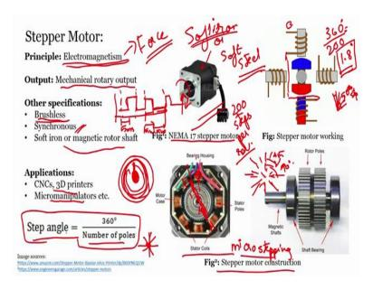
So, this is a different kind of motor as you can see in the presentation. the stepper motor is a different motor like our DC motor only you can see a stepper motor type of stepper motor named NEMA 17 stepper motor over here, You can see this black part with a black part is the body and this is the shaft that rotates,
