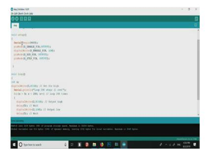
Now, inside the void setup I have started serial communication, it is not very important here I have been used it. And in the pinMode X, X should be output since it is X\_ENABLE\_PIN is output and I have made it low so that I want the motor to rotate completely I am not going to change it anyway. And pinMode (X\_DIR\_PIN , OUTPUT) (X\_STEP\_PIN , OUTPUT) you know this already,
