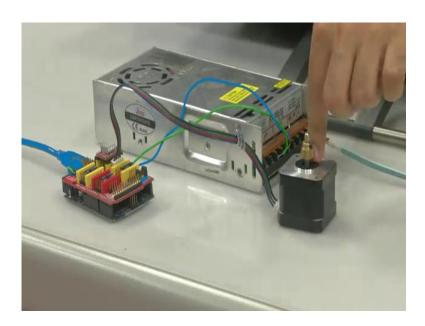
So, you can see here the stepper motor over here correct this is the NEMA seventeen stepper motor and I have got an SMBS here. This stepper motor request 12-volt power supply for it to work, so I connected an SMBS that can provide an output of twelve volts and it goes to a word over here this is an Arduino UNO board on the bottom and this is a CNC shield.
