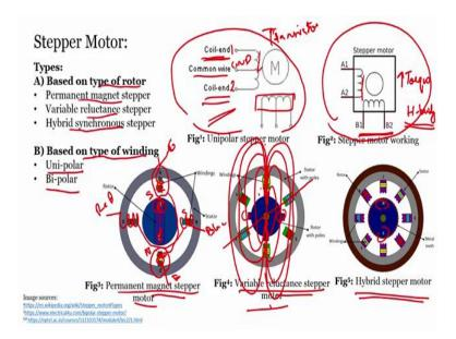
So, there are different types of a stepper motor and we classify them based on the type of rotor we can classify them as a permanent magnet stepper motor, variable reluctant stepper, and hybrid synchronous stepper, you can what do you can see here is this is the permanent magnet stepper motor; now I will tell you the concept of how it is working,
