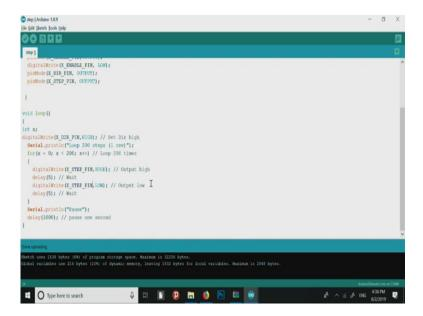
So, for creating a pulse I have used a simple method I put an integer X, I have put an integer X and digitalWrite(5, HIGH) 5 is nothing but X underscore direction pin. we already defined it
