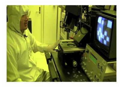
And pretty much you do is you are this controls the microscopes in the back, so you can select one at a time and move around to you find your features, it looks like we found alignment marks on the mask. We need to adjust the focus, he uses this top straight left and right, so the left one just the left you know I want to adjust the right focused.
