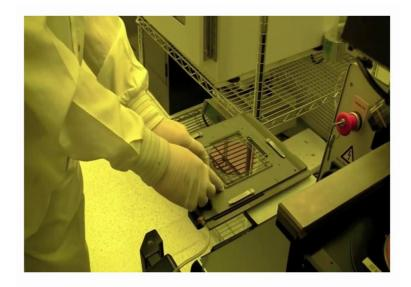
So, you load your mask in here by left in this crip here and putting it in and when it is in nice, you hit this button called enter you would toggle the vacuum. Right now the
