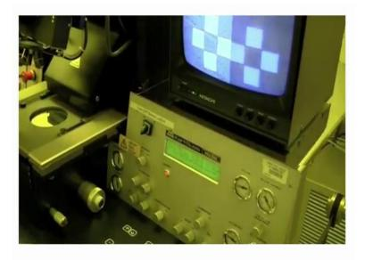
So, after exposure you need to unload wafer, so what you do is you come to the screen and you say pull slide unload expose the substrate. is pull it out and then this is you press the enter button and then the vacuum will be released. Then you can take your wafer out and then you would put it back in, so that is how you unload your weight for after exposure.
