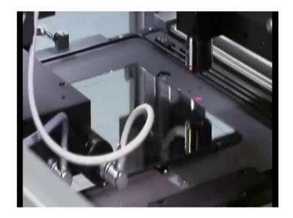
The big advantage of the steppers is the exposure of the entire wafer in one step, thus a throughput of more than 100 wafers per hour can be achieved with an overlay accuracy in the submicron range.
