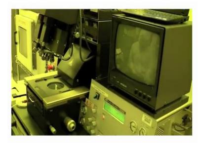
So, the first thing we do is though we have to have a mass-loaded and then we turn the screen on. Now, we make sure this thing as backside while the microscope is on it is on, but also we needed to change this to backside alignments. It can be either topside alignment or it can be a backside alignment, so this is an illumination, so now; the light is coming from the backside.
