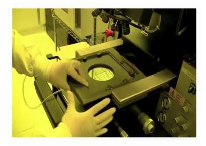
So, now we are going to put this in here, so we carefully carry it; oh, place it all the way in and when it is in the press change a mask. And that is how you load your mask when we are going to be doing a backside alignment now. What this does is it aligns features on the back of your wafer to your mask, and how you do it miss the middle microscope from the bottom.
