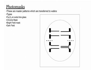
Hi, welcome to this particular module, we talked about photo mask right pause a bright field photomask and a dark field mask. This mask our master patterns which are transferred to wafers and the types of photomasks are the  $Fe_2O_3$  on soda-lime glass. It can be a chrome mask, it can be a bright field and dark field as you know.
