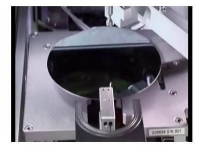
The machine runs and adjusts fully automatically and is optimized for the processing of thick resists such as with thick resist, left chip bumping, wafer-level packaging, MEMS nanotechnology or telecommunication devices.
