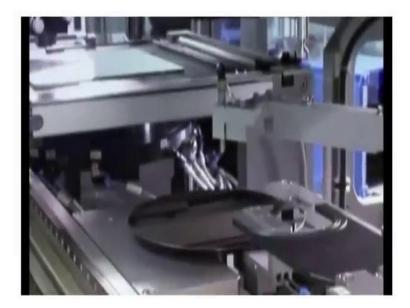
Now, let us slow the process down and take a closer look. First, the wafer is pre-adjusted onto the pre aligner in preparation for the ensuing alignment. A linear transport system loads the wafer onto the exposure chuck which together with the robot arm guarantees the optimal and flexible handling of the substrate.
