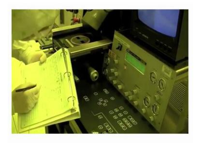
So, the compost air is about 4.9, the nitrogen is about 4.65, the vacuum is about 0.86 taking the 0.8 we use the 4-inch wafer with silicon and we did 25-second exposure. Now, I ready to turn off first what we is doing is we will turn off the switch here, also the TV screen and then we can log out here. And some messages like the do we set the x, y and tilt position now we did that, so you put.
