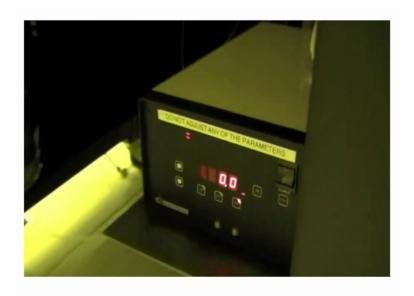
So, you check the power supply do you hold this button call the (Refer Time: 09:24) says 3 2 2 6, how many hours the bulb being used. The bulb has a lifespan of 4000 hours. when it is over 3500 we would notify staff and tell them to change it, so we are pretty close to that. Now, that the bulb is to use and that is nothing wrong with the bulb and the power supply, we want to log into the system. before we login topside we check the logbook.
