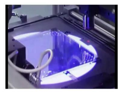
The structures of the photomask are conveyed via shadow cast, the patented wafer levelling system from SUSS compensate for topographic variations and wedge errors.
