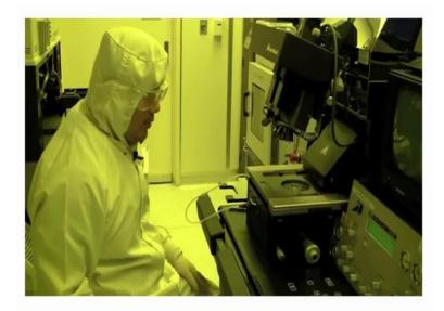
What we are going to do now is topside alignment by using the microscope on the top to align to the wafer that is underneath to the glass. to do topside alignment we need to move the backside microscope, so we press this button that turns it off, also we need it for the illumination to the top side and then now we can load our wafer pen.
