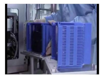
Now, I load the carrier that is all there is to it and the MA 200 compact is ready for operation. The processes of the MA 200 compact can be controlled via a touch screen.
