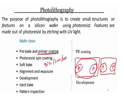
So, why we had to go for primer coating? Because the primer coating will improve the adhesion of photoresist onto the substrate. now after primer coating, you will go for photoresist spin coating. When you coat the wafer or subset with photoresist, the next step would be soft bake. Soft bake is done at  $90^{\circ}$  C for 1 minute if we are using a hot plate correctly.
