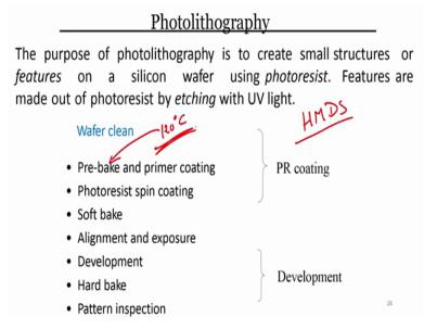
So, what is the procedure? The procedure is you have to start with the cleaning of your substrate. If it is the silicon wafer, you have to clean the wafer and then you have to pre-bake and primer coating. Your primer is HMDS. First is pre-baked; pre-baked is done at  $120^{\circ}$  C on a hot plate. a pre-baked will help to remove any moisture from the wafer, from the substrate. Then primer coating we do we coat with HMDS and then are followed by photoresist spin coating.
