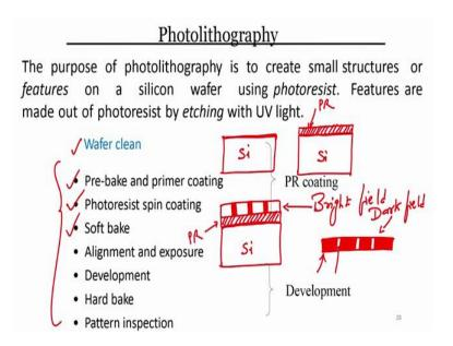
The next one is I add to align and expose. I will take my wafer, load into a photoresist UV lithography system or it is called mask aligner system. There are several mask alignment systems and then I will load the mask. this is my silicon, this is my photoresist and this is my mask. Now, the red bold area is the red this one blocks in this design are some pattern onto the mask some pattern area onto the mask.
