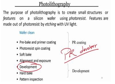
Masks are two types; bright field and dark field mask. this is about your alignment and exposure. After that, you have to develop the wafer. Developing a wafer can be done with the help of a photoresist developer, photoresist developer.
