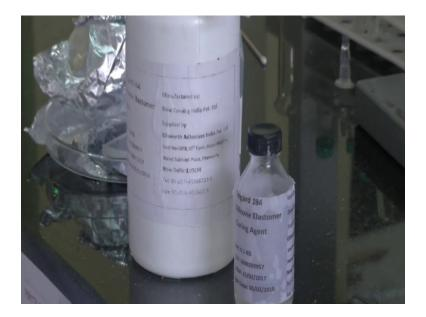
Here what I have is a silicone elastomer Sylgard 184. I am going to make the PDMS molding using this silicone elastomer, along with a curing agent. If you want to make a mould using PDMS then you might consider buying this elastomer and a curing agent. Elastomer and curing agent are mixed usually in the ratio of 10:1. When these two are combined in this ratio, a polymer is formed which can be cured and that easily. You can replicate micro to nano level features in just a few hours.
