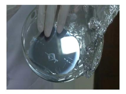
Here I have a silicon wafer. You may be able to see the fine lines here. This is embossed on the surface. This wafer has a pyramid like a rhombus structure as an embossing. You could have many different forms of this structure.
