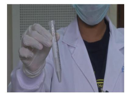
Now that I have taken some amount of elastomer, I take the curing agent. I need to take 0.5 ml of curing agent. The curing agent would be floating on top and then at the bottom I have the PDMS, the silicone elastomer. Now, we have to stir this well. You could take a stirrer and then stir them thoroughly and a lot of bubbles get formed. This process would go on in order to make the two immiscible polymers combine into a single liquid.
