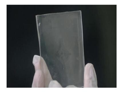
After curing the mixture at 70° Celsius for 2 hours, you get back your mould and then you could cut it using a surgical blade and this is what you get. This is the flexible PDMS substrate on which this structure was embossed.
