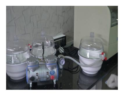
Here what I have is a desiccator. If you have not heard of a desiccator, this is a chamber that will provide vacuum. As you can see this is the top lid that is transparent and there is a bottom casing and an elastic rubber so that the lid sits tightly. You can say that this is a small vacuum chamber.
