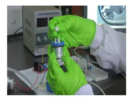
I have a peristaltic pump, like what you saw in the image previously. This is a small 12 volt peristaltic pump, I will open it up and show you how it looks like from inside. This is the flexible tube that we talked about. This will be compressed, if we give the input fluid it will be sucked and pushed in and the output will come through another tube using nothing but just a DC motor here.
