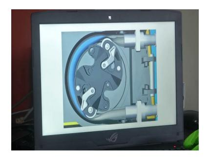
Now, I will show you how a peristaltic pump works. you can see here in a GIF image that the fluid will come through a port. What we have is a rotating a roller kind of thing and in that rotating a roller itself we have some small different wide rollers.
