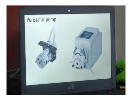
On the screen, you can see two pumps, one 12-volt peristaltic pump and another costly peristaltic pump for the microfluidic application. You must have seen this kind of peristaltic pump as a part of the lab videos. These peristaltic pumps are positive displacement pumps and they are used for very precise applications especially in micro fluidics, drug delivery and other things where the flow has to be controlled very accurately.
