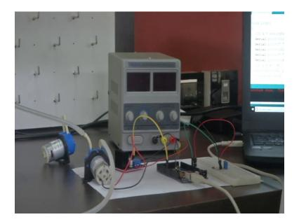
as we can see it is the same circuit that we used previously. I have the mega board, I have the potentiometer connected, I have the motor driver 1 2 9 8 10 and the peristaltic pump I showed to you. And then here is a peristaltic pump that is connected to the circuit in the same way as the motor driver was, the motor was connected to it. There is a DC motor in the peristaltic pump, and the tubes.
