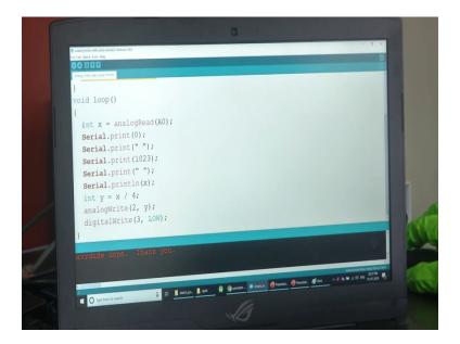
The same process in which we took the analog value from the potentiometer and printed it. On the serial plot plotter the value y will be stored with the value of x / 4. We can adjust the range from one 0 to 10232, 0 to 255 then using the analogWrite (2, y), I am controlling the speed of the pump and here it is ground, in other terminal of the pump.
