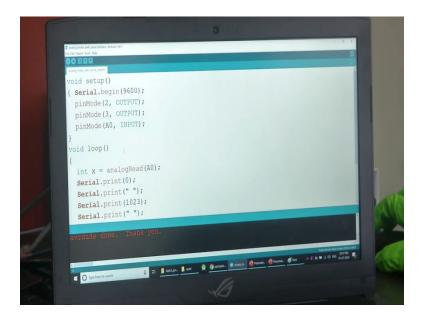
You may remember this Arduino code. It is the same code that we used for the motor. I have used the serial communication, then pin number 2 and 3 are connected to the motor driver, over here it is the pump that is being connected to the motor driver now and I have connected a potentiometer to the analog pin A0.
