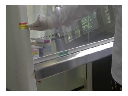
The sash line has been designed to protect the person from any contamination.
