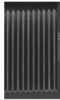
cross section of a silicon wafer demonstrating trenches that can be fabricated using DRIE tech
