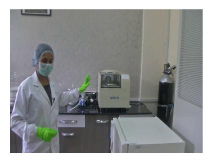
There are two types of incubators in the lab the shaker incubator and the static incubator. to maintain thus you have two levels of temperature and humidity depending on the sample for the appropriate growth of these samples have a shaker incubator where the samples are being vibrated at a certain rate and can set RPM.
