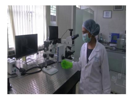
There we have a stereomicroscope and a metallurgical microscope. So, again the choice of microscope for your study becomes important when you are talking about silicon chip
