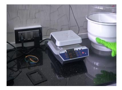
Here we have the hot plate with a temperature closely temperature control system, a magnetic vibrator as well. And why do we use the hot plate; again, an important step during the microfabrication process, soft baking. Every time you pin coat, you will have to bake and that is when you use the hot plate in order to remove the dissolved solvents in the photoresist that use pin coated. So, for that purpose, we have a hot plate here and then comes the microscope.
