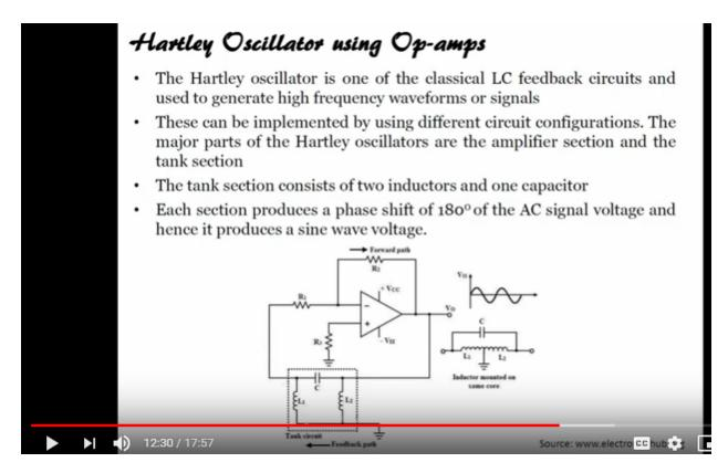
Now, if I want to design hudley oscillator, if I want to design hardly oscillator, then this is the way to design hardly oscillator, this is a tank circuit as we know Right? And this can be implemented by, by using two inductors and, one capacitor each section produces a phase shift of 180 degree Right? Each section produces 180 degree and, hence it produces a sine voltage Right? And produces a sine wave voltage.
