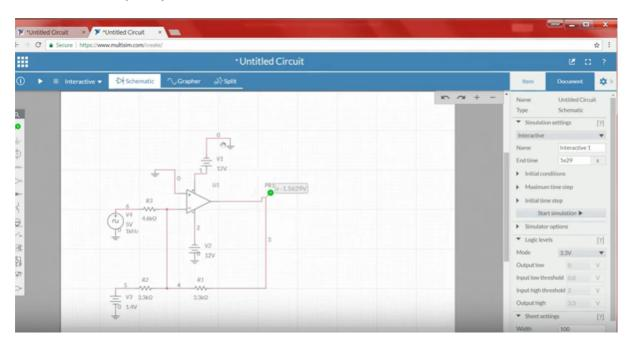
Now what do we do, in order to get, the positive voltage, like I'd mentioned, just give the feedback that is the output of this, will again be, feedback to the similar circuit and that is when, you will be able to get the desired, output voltage. Okay? Let's give the output, of this to the same circuit, now I leave that, to you, on the similar basis, connect the output voltage to the similar circuit, so you could work on, the circuit, what add mentioned? And you could also
