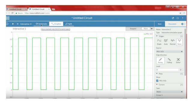
the desired voltage that is from positive 1.4 to 5 volts. So this is how, you can generate, signals or of desired, voltage level, based on the requirement of your sensor or depending on different applications,
