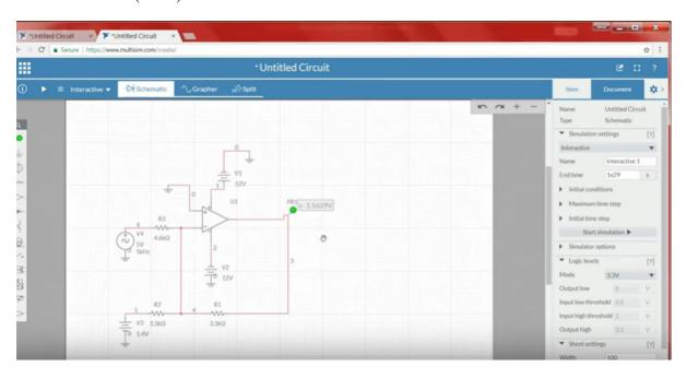
So, this was a basic simulation, about how you can choose, the different source the input source voltage, like your function generator, it plays the role of your function generator and how you can rig up the, circuit using the multi-sim, even before you, get into the hardware. Now, go ahead and give the output of this to the feed, the output of this to the similar circuit. So that, in your graph you observe
