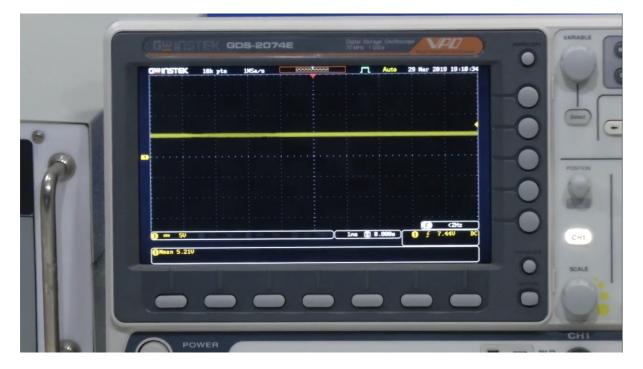
Now the voltage difference once I removed, so now that I have the icepack close to the heater, you see the difference in voltage. As I get it back, let's see how sensitive our op-amps or the device, the Pt100 sensor is. So when I have the icepack close, let's see how quickly it would rise. The change in voltage can be observed from the CRO. So now 5v, so as you see the voltage is rapidly increasing.
