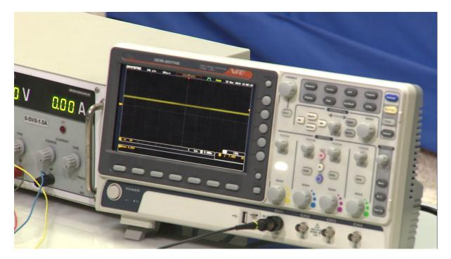
Now for steady state without flow let's see what is the output voltage. Looking at the oscilloscope here, here you can see the set voltage of 5v and here the voltage across sensor that is the Pt100 is showing 4.8v which is close to your set value. Now what happens when air flows through your Pt100.
