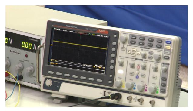
So when I cool, assume there is air flow and is taking away the heat from your Pt100, the voltage varies. So you see the voltage is going up to 5.6v. So we have a reference voltage which is 5v, the differential voltage is rapidly increasing. So now it is 5.48.
