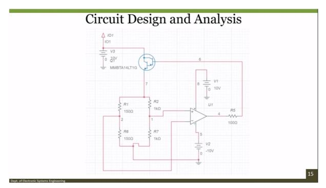
So as I mentioned the bridge connection is like this, like we have the heater here, the Pt100 if that becomes the portion where the sensor where you want to integrate this with the anemometer. So your sensor would come here. This is a series resistor, 150 ohm series resistor and R7 would be your temperature compensation resistor and then in series is your 1 kilo ohm resistor.
