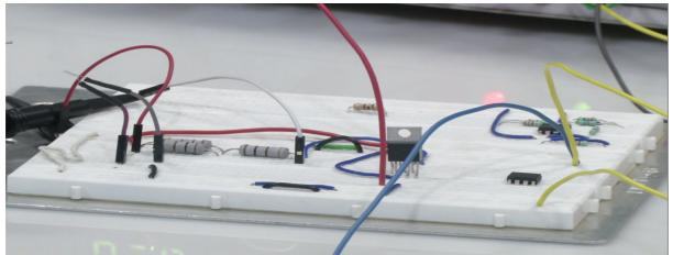
So initially this is the circuit what the board you see here. So the two resistors here are 100 ohm, this is 100 ohm, and the two connected in parallel, 50 ohm. So this net R value, 150 ohm if connected in series with the tiny Pt100 what you see here, the blue small chip here is nothing but your Pt100 sensor and then we have connected instead of giving the compensatory circuit, we have given a constant reference voltage through the circuit.
