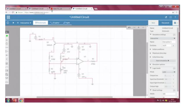
Getting to the details about the simulation; so initially let's construct the bridge circuit. So I'll take the four arms of the bridge and then the change the resistance, let's take one 150 ohm here, and then the same thing here. Let's assume we have the platinum resistor here which is the other arm of the bridge and here, one this end, if I have mentioned in the previous module, we need a higher resistance on the other arm of the bridge.
