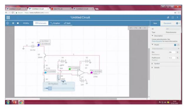
Now assume, I am going to change the compensatory circuit here assuming the room temperature is increased to 50°C. So what does my table here tell? At 150°C, it is around 157.33. Now how do I simulate that condition here?
