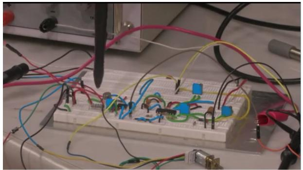
as you have already seen when we are working with a motor, so this is our motor which we have also used in the last sessions when we are discussing about DC motor, when we are looking about the working of encoder that time we've also seen the same motor which is DC gate motor and with encoder connected together.
