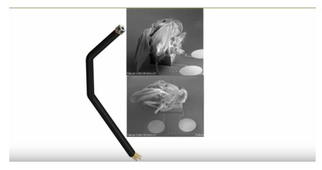
So, if you see the screen, what you see here is a, 3d maps based strain gauge or at the tip of the catheter.
