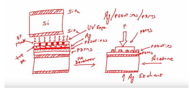
What you want to have? You want to have, P DMS bump on the strain gauge. So that, this bump will help us or will facilitate, the force that we apply on the strain gauge to, to transfer the force that we apply, externally to the strain gauge, alright. So, PDMS bump, how can we create this PDMS pump? For creating this PDMS pump, we have to perform again a lithography.
