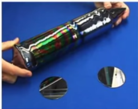
Wafers are cut from boules , which are large logs of uniform silicon.
